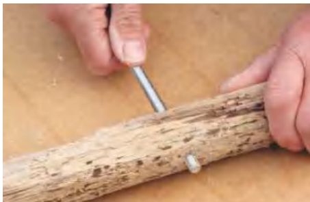
▲ Pic.4 The studding should be a tight fit in the bottom branch. Enlarge holes in the remaining wood if necessary
